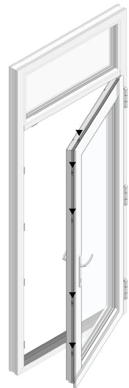
Figure 7 - Black rectangles indicate CAM locations on this unit (may vary on other models)
