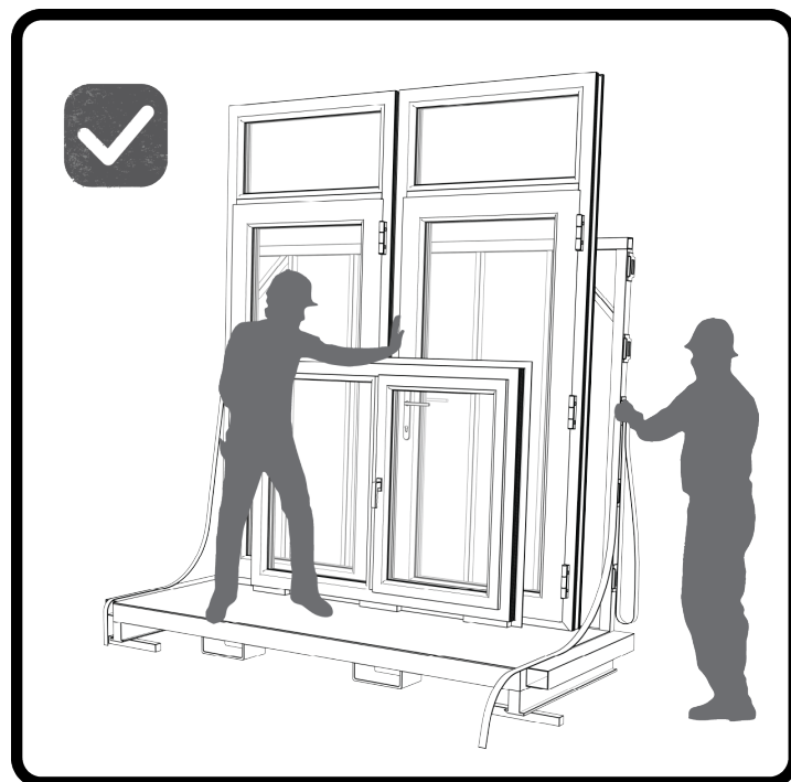
Figure 2 - With two+ people, remove straps one at a time, starting from the front.
