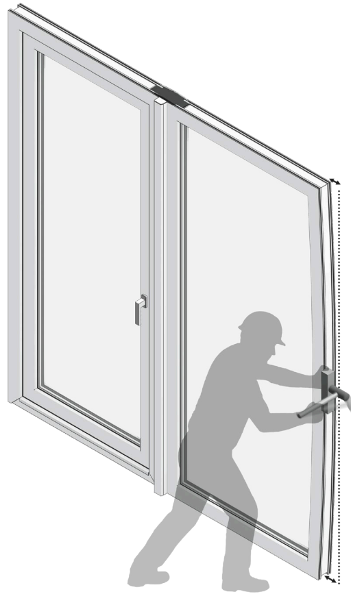
Figure 45 - Tapping Frame Back into Alignment
