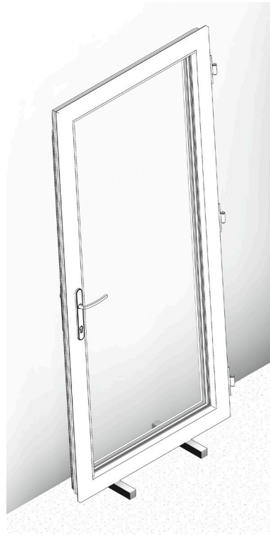
Figure 17 - Storing the Sash on Support Blocks
