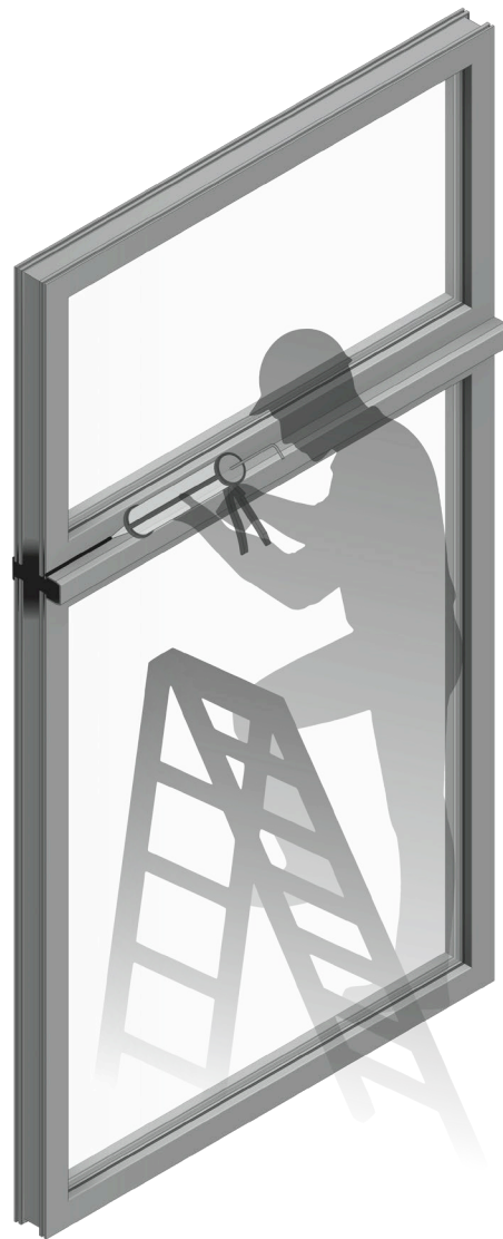
Figure 74 - Sealant Bead at Horizontal Coupler
