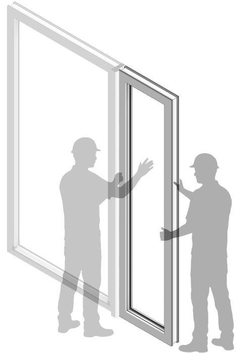
Figure 70 - Frame Seating Evenly on Coupler Shims
