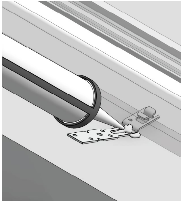
Figure 28 - Apply Sealant to Anchors
