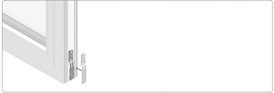
Figure 48. Placing the anchor into the groove.
