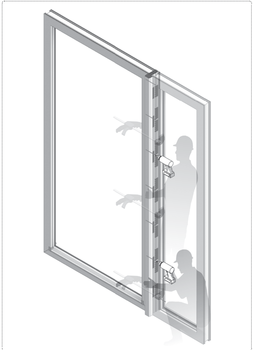
Figure 71. Screwing frame to coupler at pre-drilled holes.
