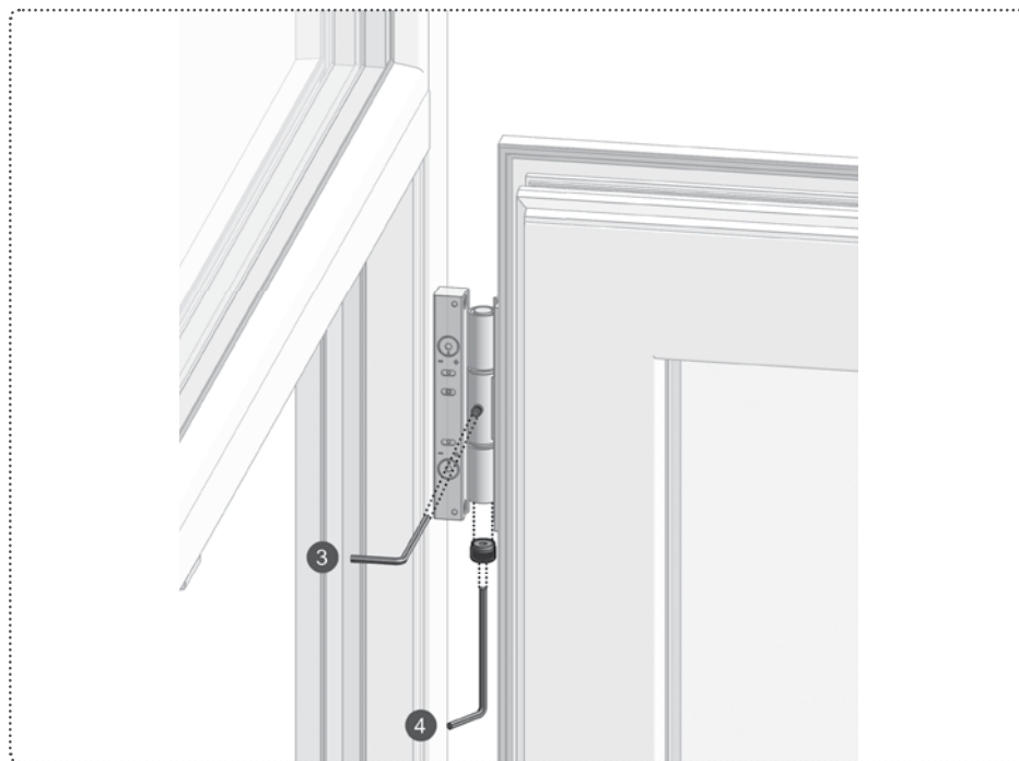
Figure 13. Removing hinge adjustment bolts.
