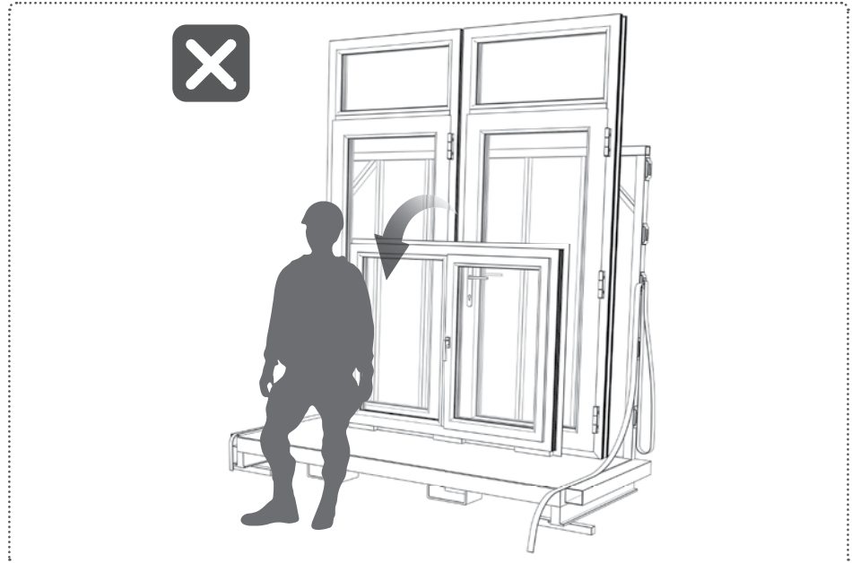
Figure 1. Never leave product unsecured or unattended on the steel rack.
