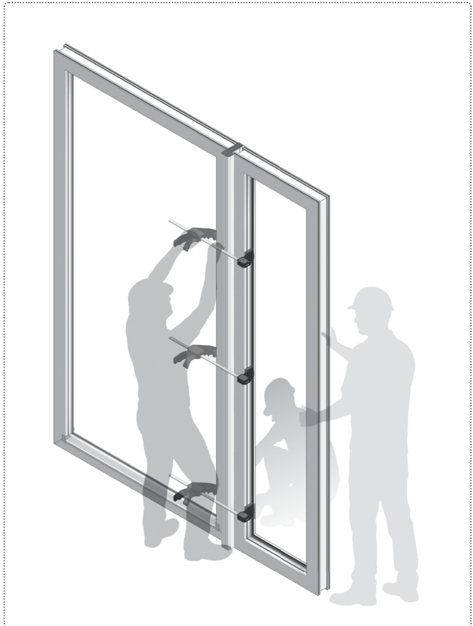
Figure 70. Evenly clamping frame to coupler.
