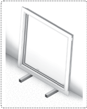
Figure 6. Sash placement on support blocks.
