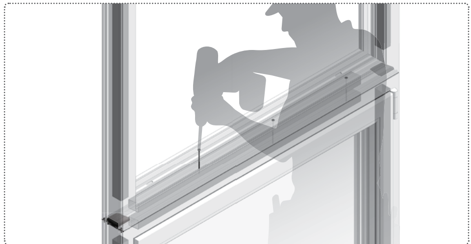
Figure 75. Coupling frames and securing with screws.
