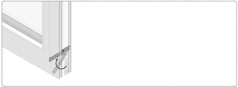
Figure 49. Turning the anchor clockwise 90°.
