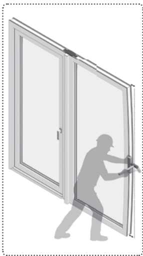
Figure 17. Tapping frame back into alignment.
