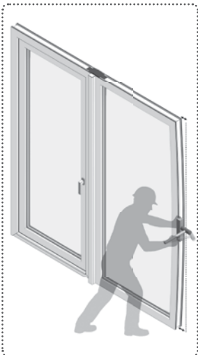
Figure 46. Tapping frame back into alignment.
