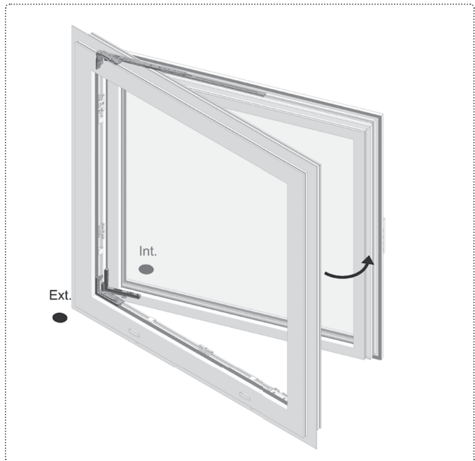
Figure 8. Opening window to access stay arm.
