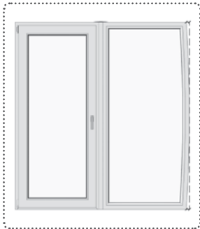
Figure 16. Bowed frame condition (illustration exaggerated).
