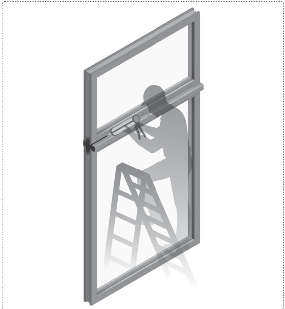
Figure 72. Sealant bead at horizontal coupler.
