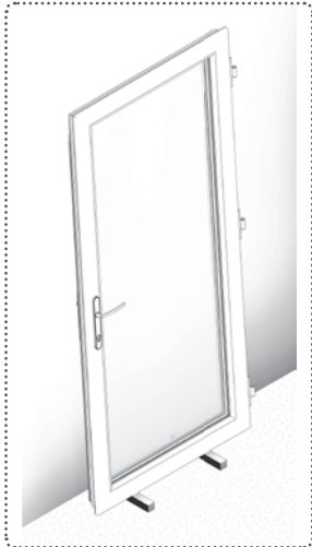
Figure 15. Storing the sash on support blocks.
