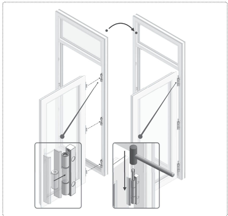
Figure 63. Installing side-hinged door sash.
