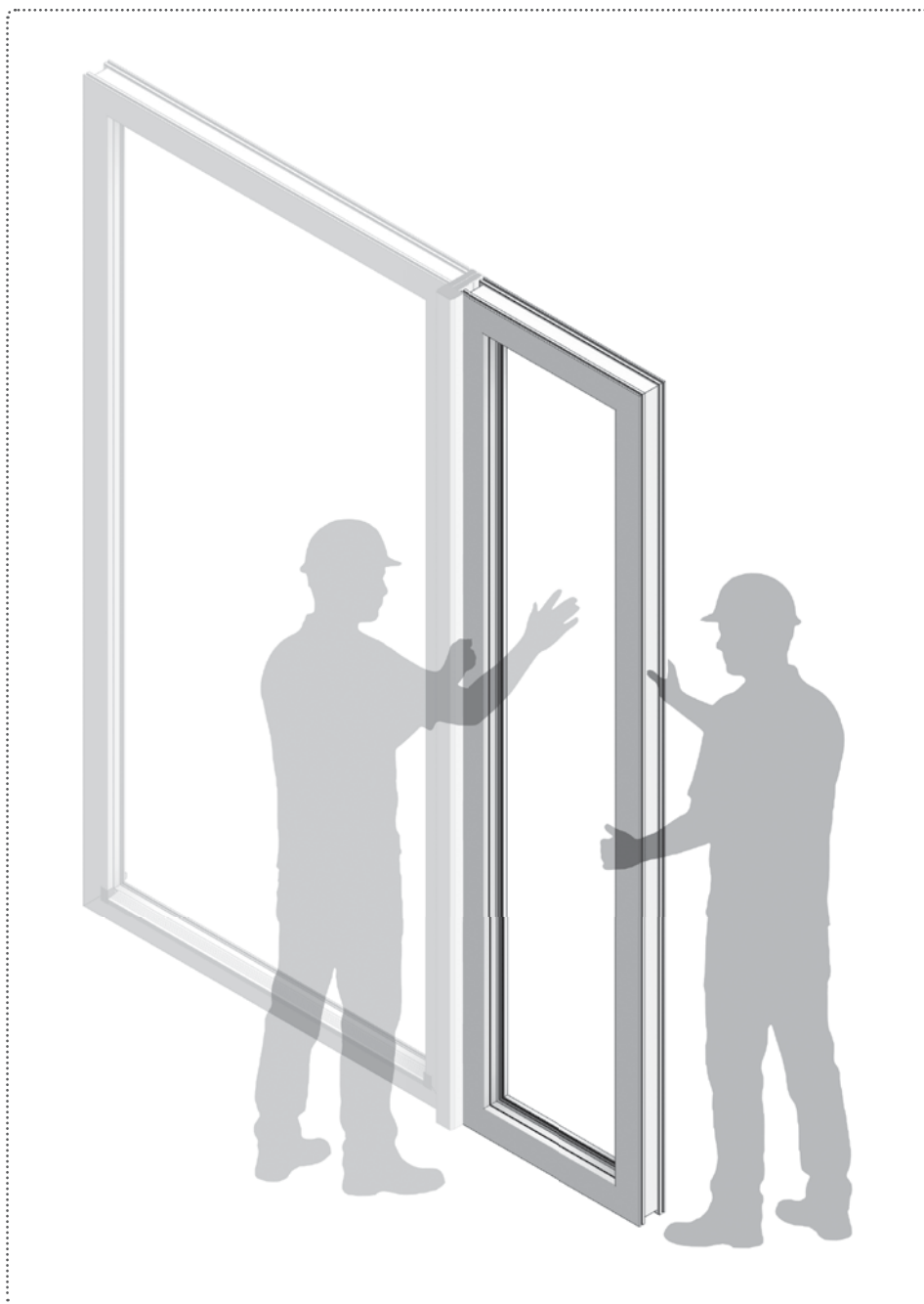
Figure 69. Frame jamb seated evenly on coupler shims.
