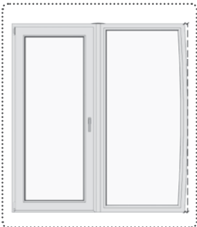
Figure 45. Bowed frame condition (illustration exaggerated).
