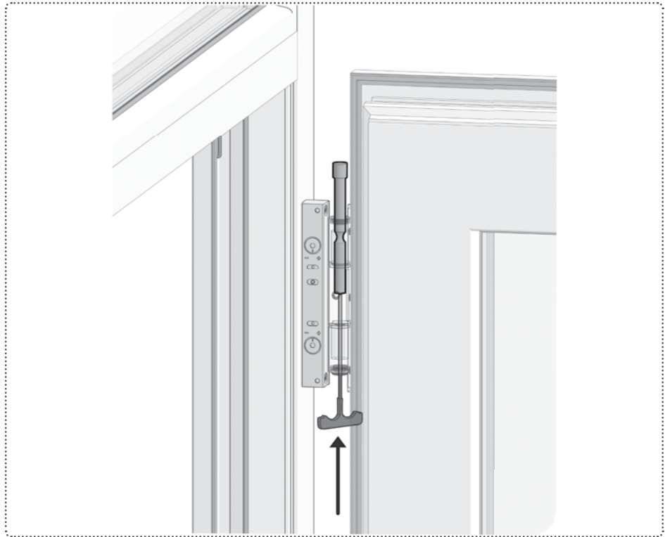
Figure 14. Removing door hinge pins.
