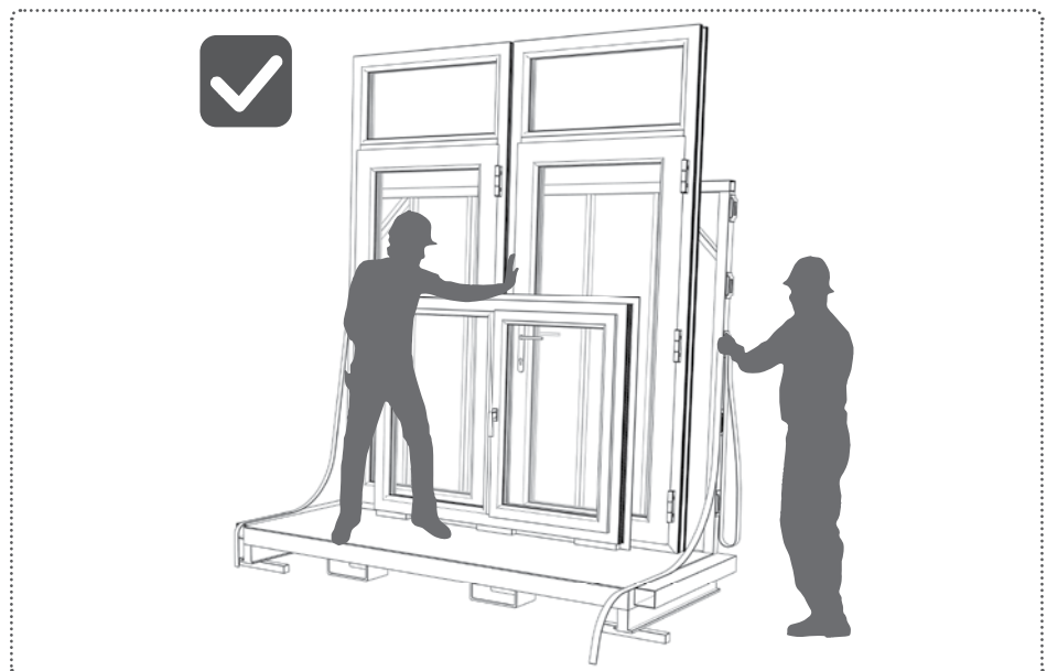
Figure 2. At least one person should hold the products while the other slowly loosens and removes the ratchet strap.
